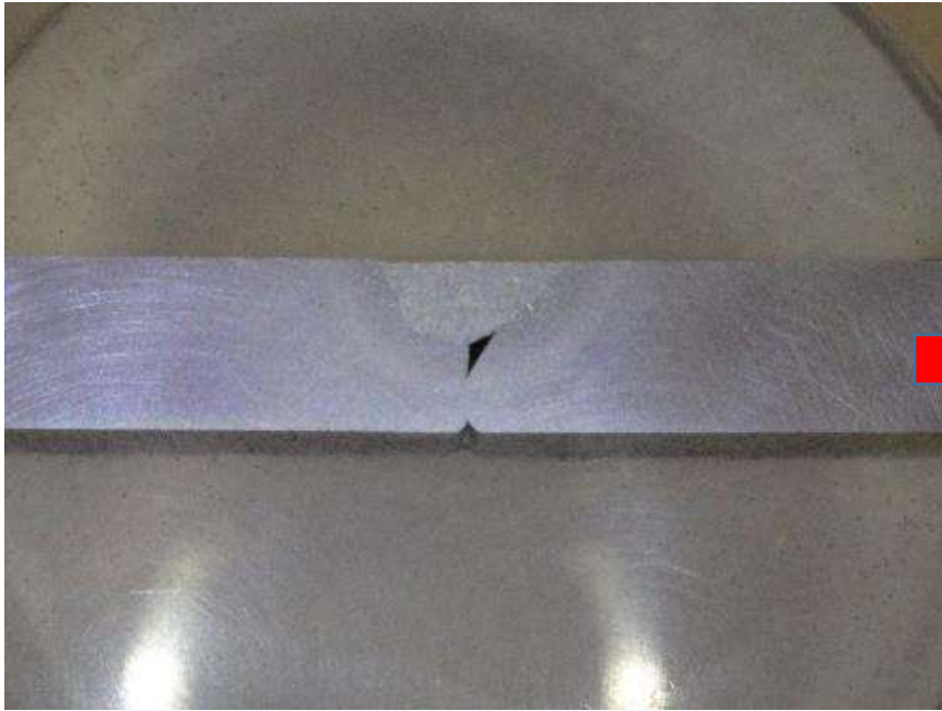
Figure 1: A36 mild steel welded with ER70S rod. Etched with 5% Nital (1st stage).
