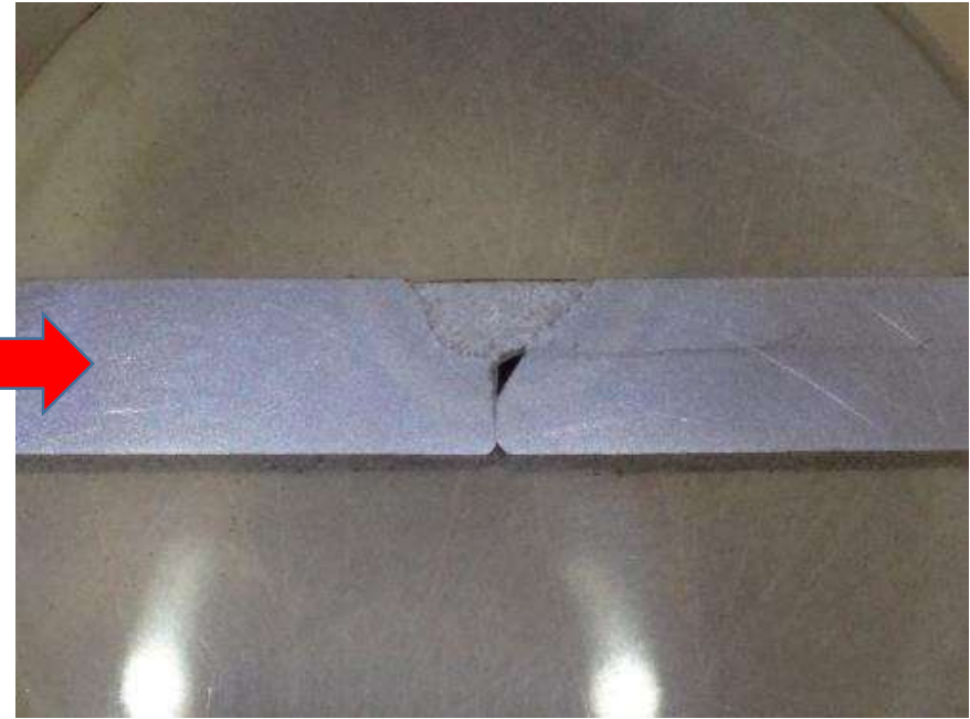
Figure 2: A36 mild steel welded with ER70S rod. Etched with 5% Nital, cleaned, dried, and then re-etched with Fry's reagent (optional 2nd stage).
