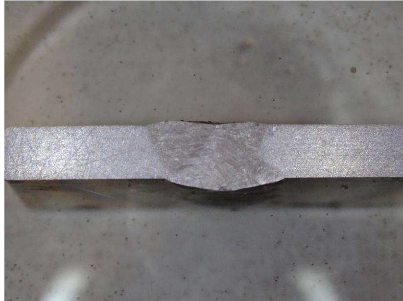
Figure 2: Welded 308 stainless steel plate. Etched with Stainless steel weld etch. The surface was mirror-polished.
