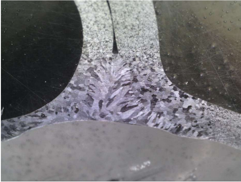
Figure 9: Welded 409 stainless steel part. Ground with 600 grit sand papers then etched with Stainless steel weld etch. This picture was taken with a handheld digital microscope and a ring light.
