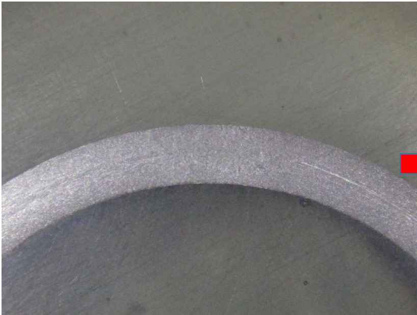
Figure 5: Welded 17-7 PH stainless steel pipe. Ground with 600 grit sandpapers and then deeply etched with Stainless steel weld etch for at least 1 minute.
