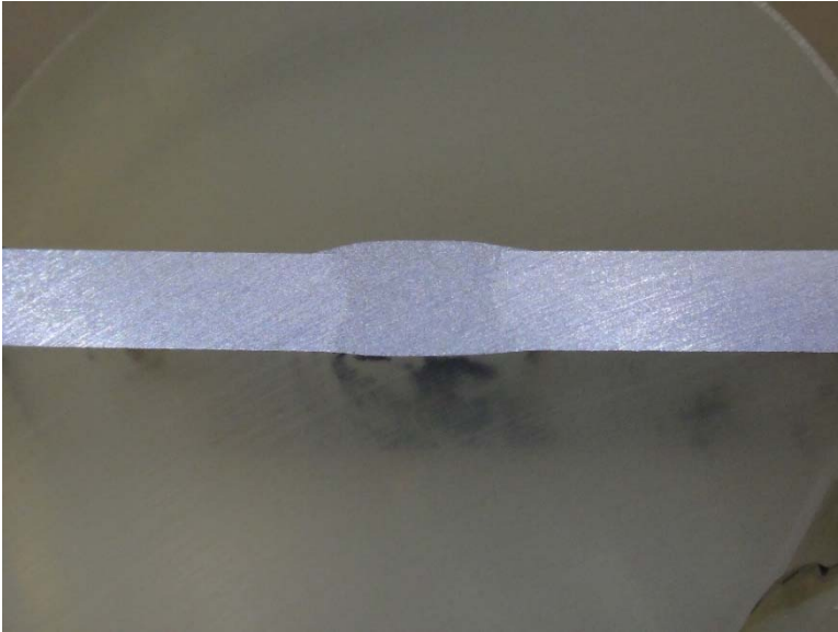
Figure 1: 6063-T52 aluminum plate welded with ER4043 rod. Ground with 600 grit then etched with the Caustic etching solution.
