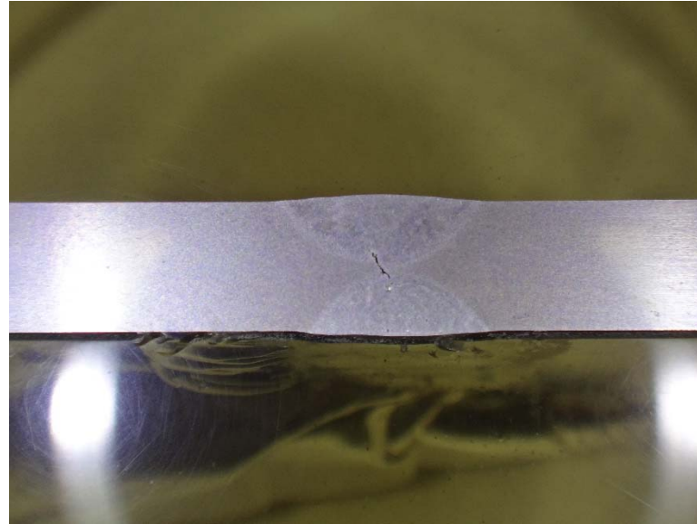
Figure 6: 6061-T6511 aluminum plate welded with ER4043 rod. Mirror polished then etched with the Caustic etching solution.
