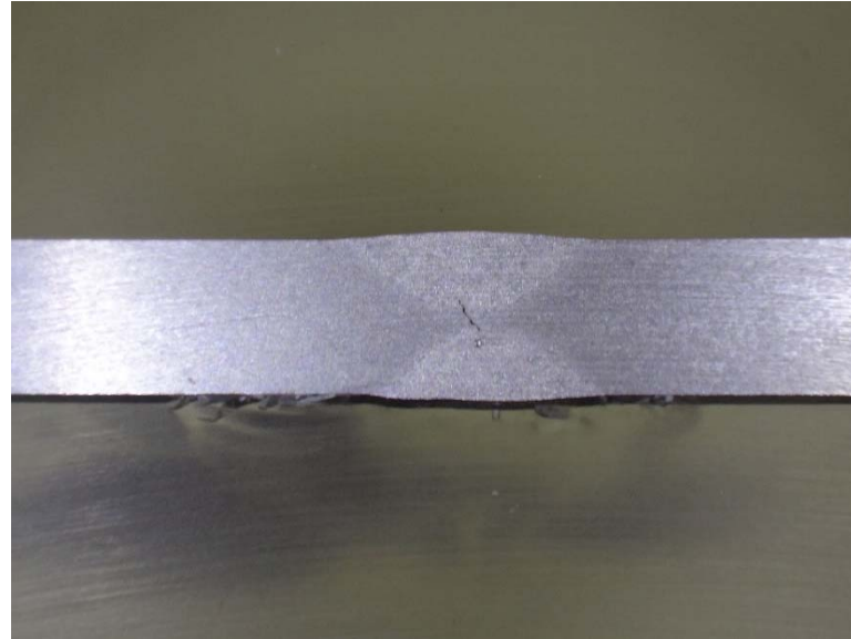
Figure 2: 6061-T6511 aluminum plate welded with ER4043 rod. Ground with 600 grit then etched with the Caustic etching solution.
