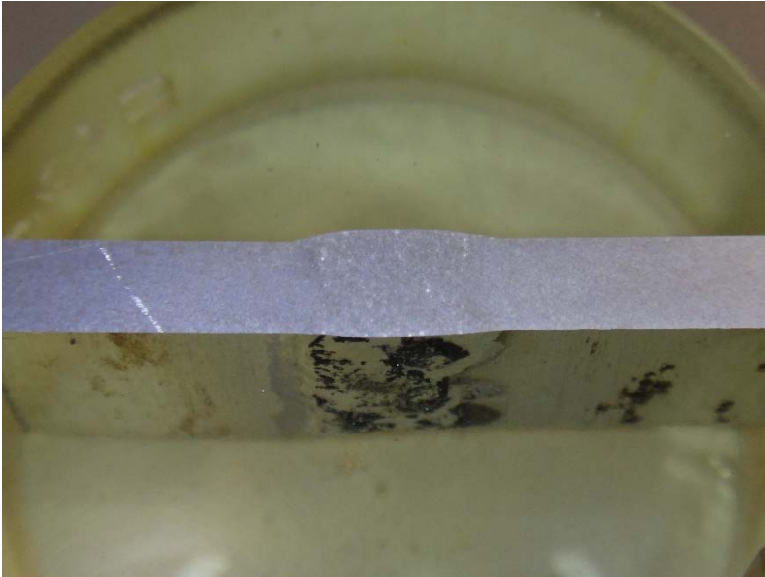
Figure 5: 6063-T52 aluminum plate welded with ER4043 rod. Mirror polished then etched with the Caustic etching solution.
