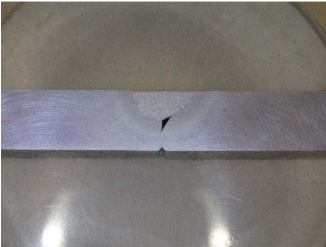
Figure 1: A36 mild steel welded with ER70S rod. Etched with 5% Nital etch (1st stage).
