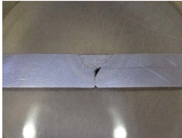
Figure 2: A36 mild steel welded with ER70S rod. Etched with 5% Nital etch, cleaned, dried, and then re-etched with Fry's reagent (optional 2nd stage).
