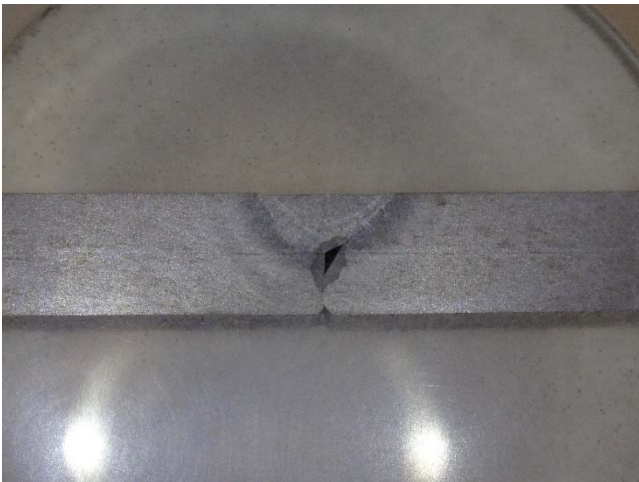
Figure 3: A36 mild steel welded with ER70S rod. Etched with the Ammonium Persulfate Solution only.
